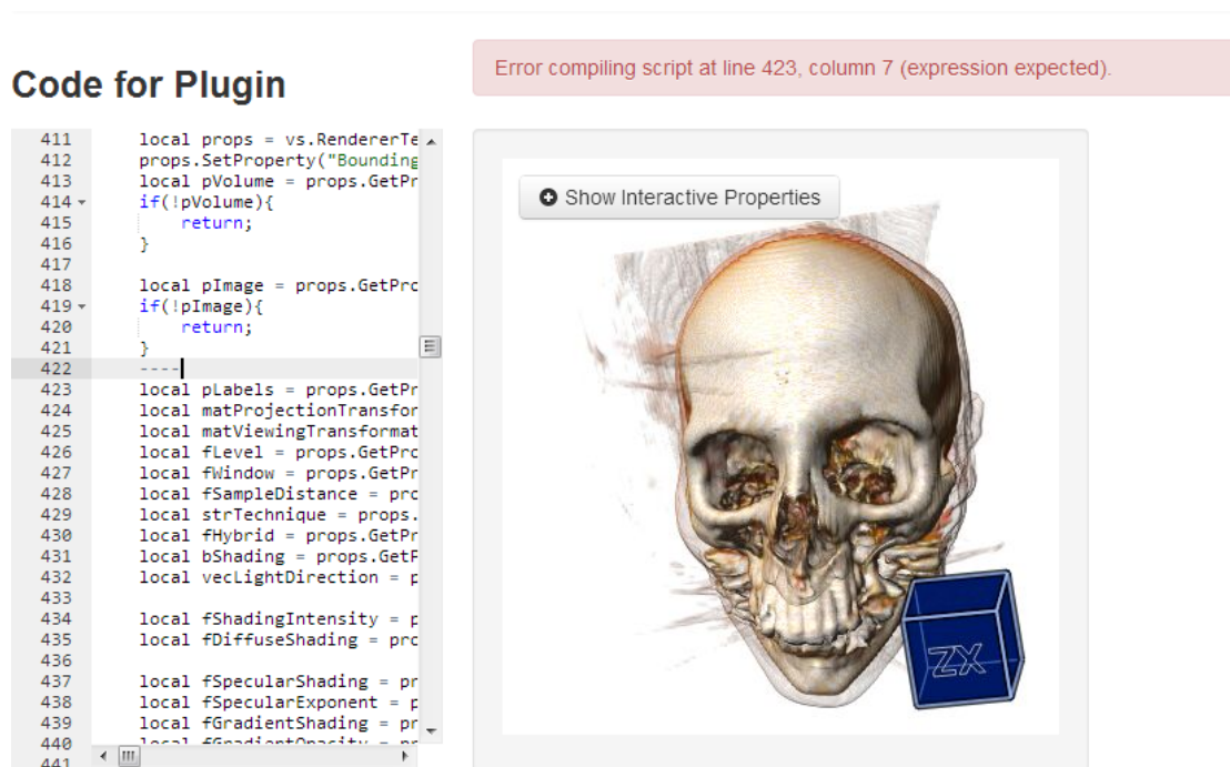
Figure 4.1: Compiling an erroneous script will result in an error message showing the line, column and a hint regarding the compilation error
