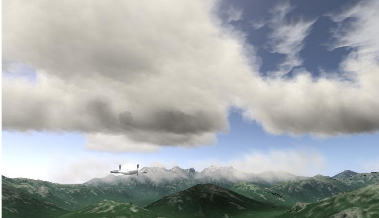
Figure 1: CloudyDay: Rendering of 3D clouds (stratus, cumulus clouds at center), 2D clouds (stratocumulus clouds at top) atmosphere, terrain, and airplanes to test Computer Vision (CV) algorithms.
