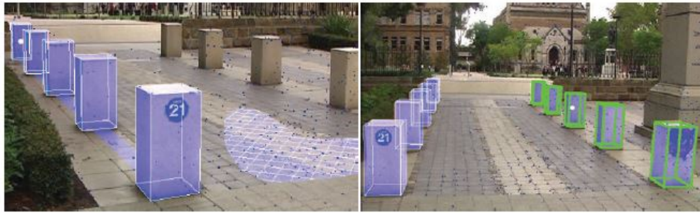
Figure 2.4: Image-based modeling for videos. Objects like the bollard can be reconstructed and replicated, as depicted in the left image. The right one illustrates replication of a whole group of objects. Image taken from the work of Hengel et al. [vdHDT + 07].
