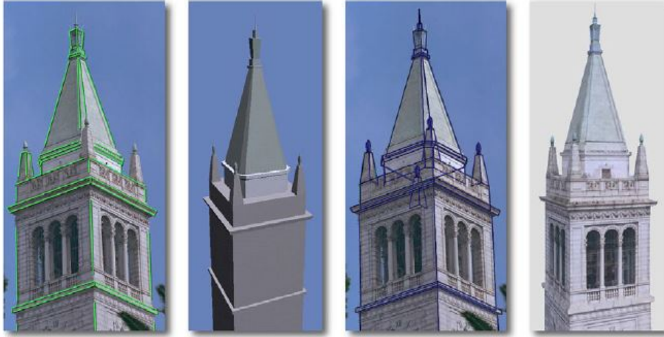
Figure 2.2: Example for image-based modeling. Photos are used to sketch the outlines of shapes, which form objects in a 3D representation. This method can also be used to define regions for later texturing. Image taken from the work of Debevec et al. [DTM96].
