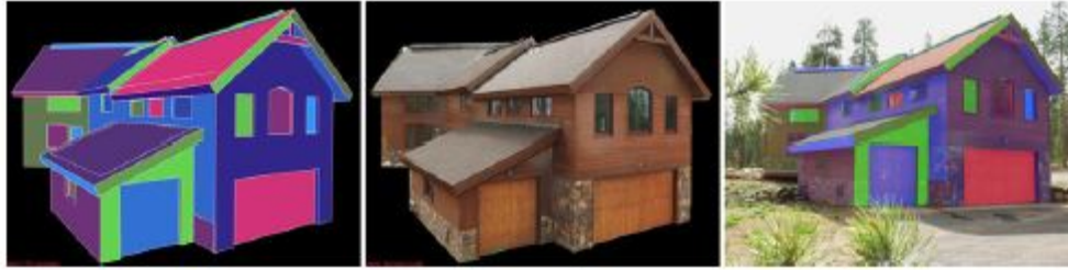
Figure 2.5: The combined approach for modeling and texturing in 1 step. The user defines shapes according to the differently oriented segments in the image, which are transformed into textured surfaces. Image taken from the work of Sinha et al. [SSS + 08].
