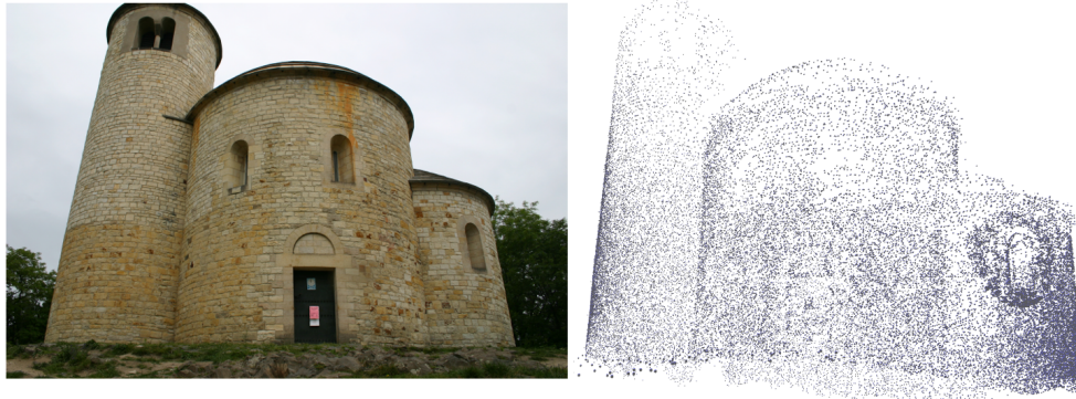
Figure 1.1: A photo of the St.George dataset [STG] and the corresponding 3D point cloud viewed from the same angle.
