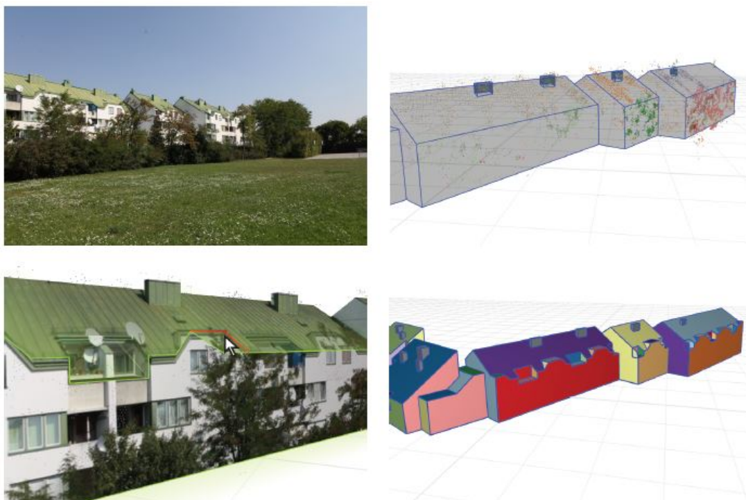
Figure 2.30: Example for an entirely reconstructed dataset of a building (photo on top left). Taking a sparse point cloud the reconstruction of a simple model was possible in 3 minutes (top right). Image reprojection onto the model helps the user to create and adjust fine details (bottom left) and create a more sophisticated model in 20 minutes (bottom right). Image taken from the paper of Arikan et al. [ASF + 13].
