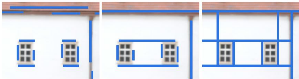
Figure 2.20: Merging of nearly collinear line pieces (left) to bigger segments (middle). The grid is constructed by extending each line until it intersects with another one. Image taken from the dissertation of Reisner-Kollmann [RK13].
