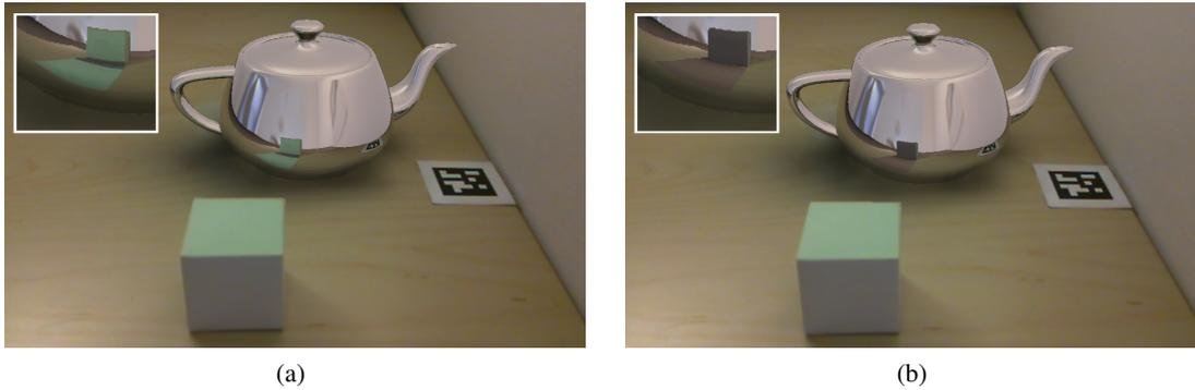
Figure 4.14: The green top face incorrectly appears in the reflection of the teapot (Image (a)). A depth comparison detects these errors and therefore uses the data from the buffer  $L_{rv}$  (Image (b)). Also note the missing back-projection data in the field of view at the border of the desk appearing in the reflection.
