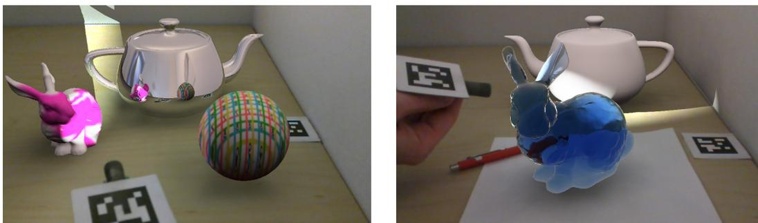
Figure 4.1: Reflections and refractions in a mixed reality environment. In Figure (a), the differential rendering effect is also applied to the real desk in the reflection of the virtual teapot. In Figure 4.1b, the virtual Stanford bunny refracts real and virtual objects.
