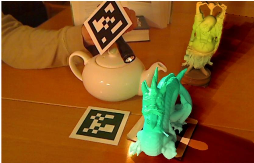
Figure 2.7: Output image, created with the RESHADE framework. The spotlight illuminates the virtual Stanford dragon that causes a green color bleeding on the real teapot. The markers are used to identify and track the position and orientation of the objects. Image courtesy of Knecht et al. [22]
