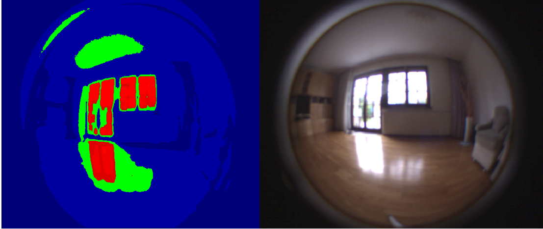
Figure 3.2: The left image visualizes how the images are combined to one HDR image. The green pixels are the pixels taken from the first image of the loop, the red pixels are from images taken with a lower exposure time which cover the bright areas, the blue pixels are from the images with higher exposure times which cover the dark areas. The brighter the color, the lower the exposure time and the higher the luminance of the scene. The right image is a picture of the scene taken with the same exposure time as the first image and should serve as a reference.
