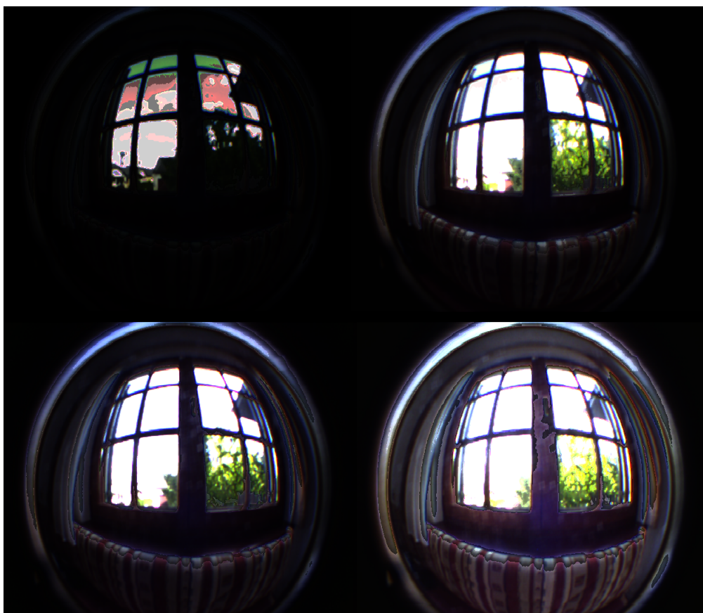
Figure 5.6: A HDR image of the view out of a window. It was displayed using the formula \log(\text{multiplication factor} * \text{pixel color value} + 1) and the multiplication factors 5, 25, 50 and 100.
