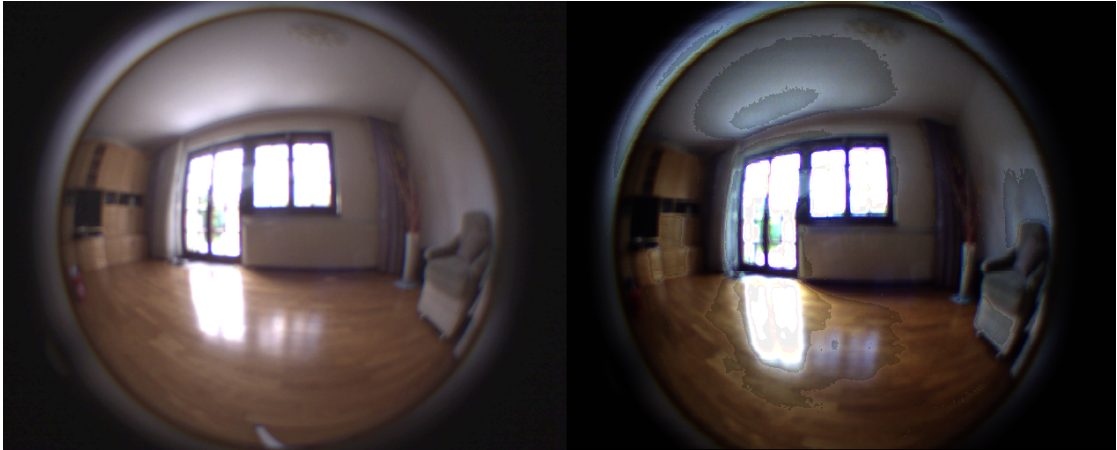
Figure 5.1: A comparison between a single picture taken with the exposure time 16 ms on the left and a HDR image display with the formula \log(50 * \text{pixel color value} + 1) on the right.
