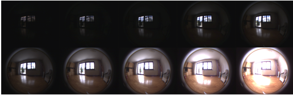
Figure 5.3: A sequence of images used to calculate the HDR image in figure 5.2. The images were taken with the exposure times of 0.125, 0.25, 0.5, 1, 2, 4, 8, 16, 32 and 64 ms.
