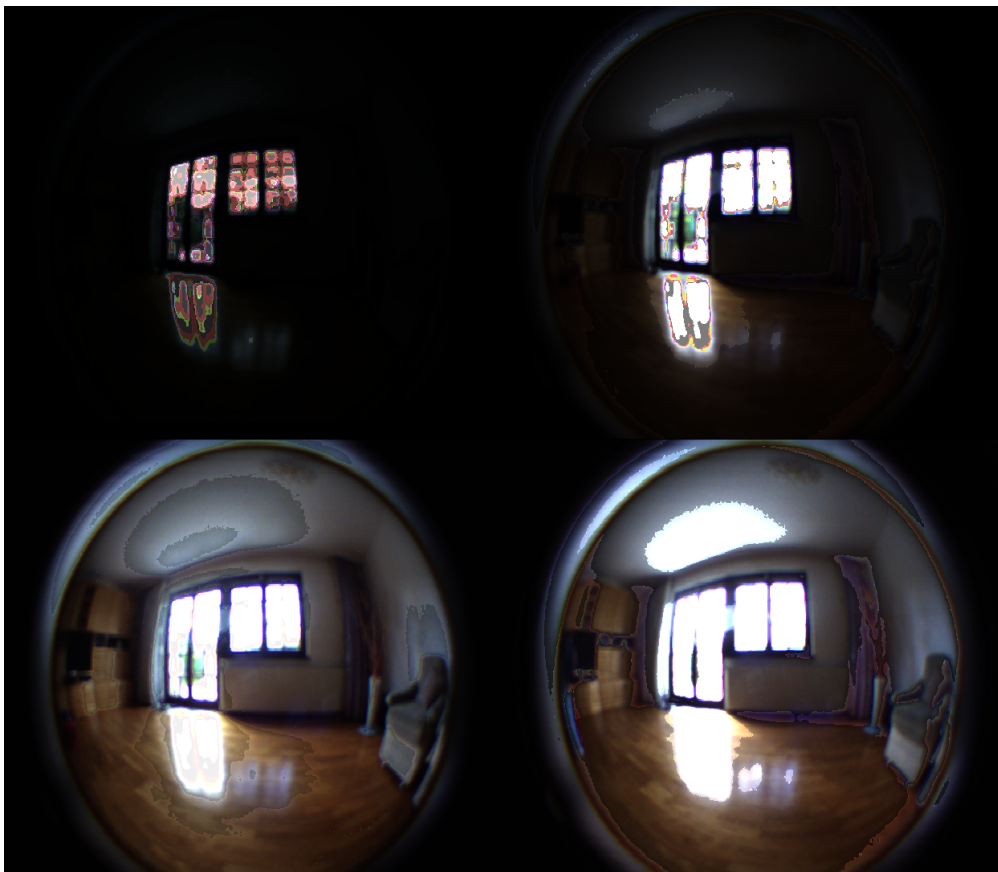
Figure 5.4: A HDR image of a living room. It was displayed using the formula \log(\text{multiplication factor} * \text{pixel color value} + 1) and the multiplication factors 1, 10, 25 and 50.
