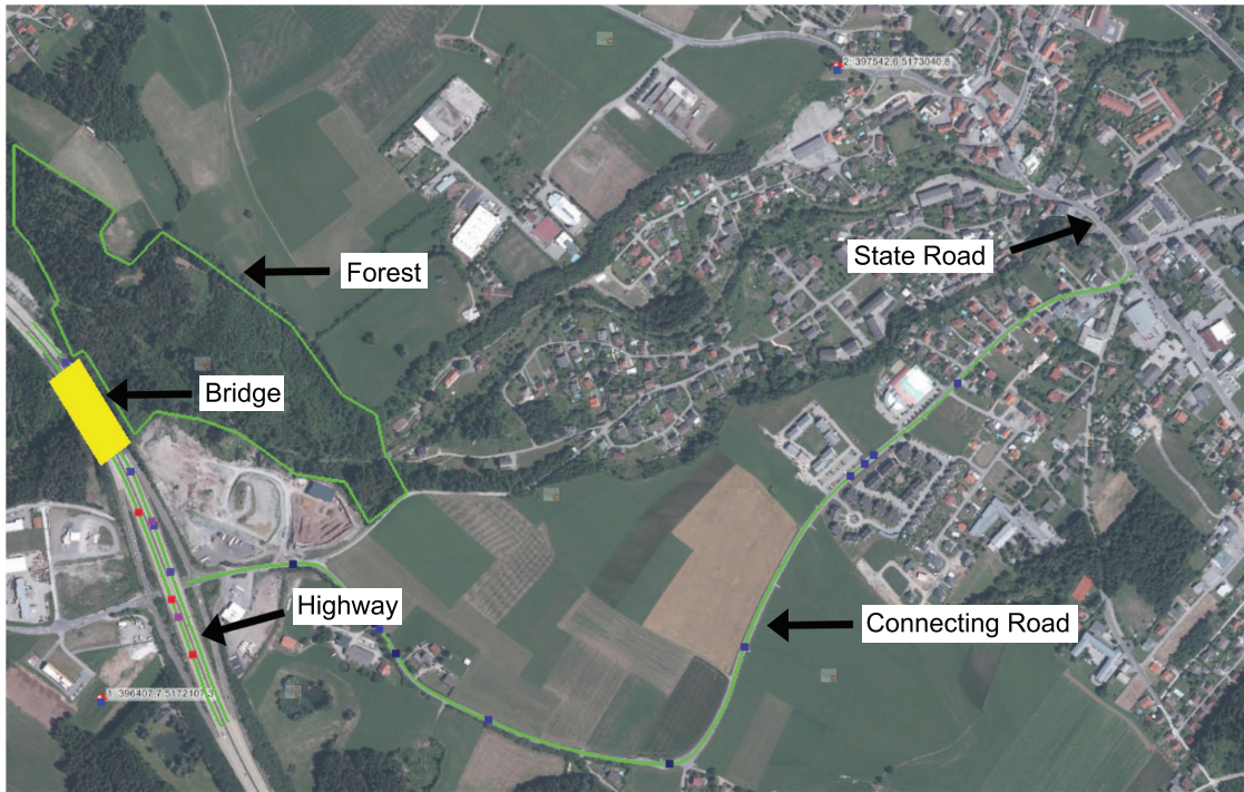
Figure 6.4: 2D view of the current traffic situation in Canyon Village. Since for the immission point of this scenario background noise is dominated by the highway traffic, other streets and emitters can be safely ignored and are not shown or simulated separately. The green polygon outlines the relevant part of the forest. The yellow rectangle depicts the location of the bridge across the canyon.
