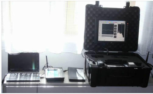
(a) Sample long-term measurement setup consisting of a weather station (to the right of the laptop, sensor outside) and a standardized sonar, in this case a 01dB Type Symphonie (in the suitcase, microphone outside).
