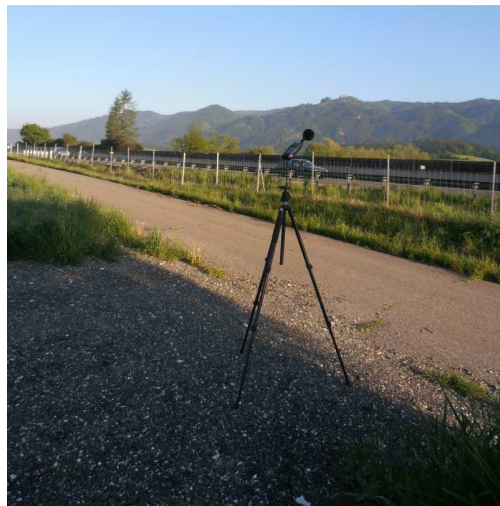
(d) Noise emission measurement of vehicles on an Austrian highway at a distance of 19 meters. Results can be found in Figure 6.7.
