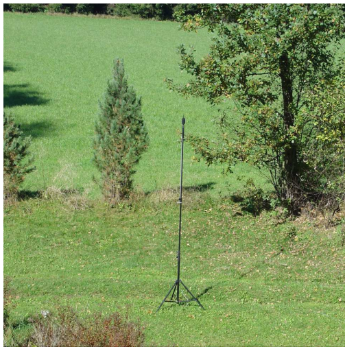
(c) Outdoor placement of a standardized sonar. To avoid reflection biasing, the microphone needs to be set up apart from buildings and other structures.
