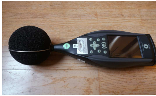
(b) Close-up of the Brüel & Kjaer 2270 Sound Level Meter.
