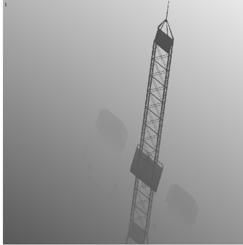
Figure 2.1: Shadow map consisting of depth values determined from the light’s point of view
