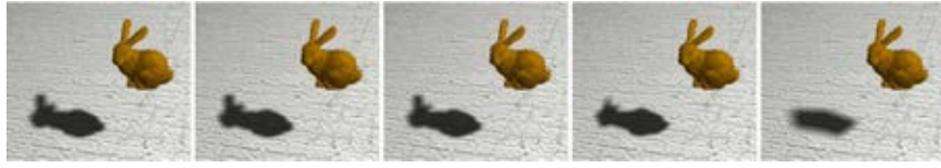
Figure 2.1: Sattler et al. could show that in case of the Sanford Bunny model 1% of the original number of triangles was sufficient to produce realistic soft shadows for 90% of the tested persons. (Source [40].)
