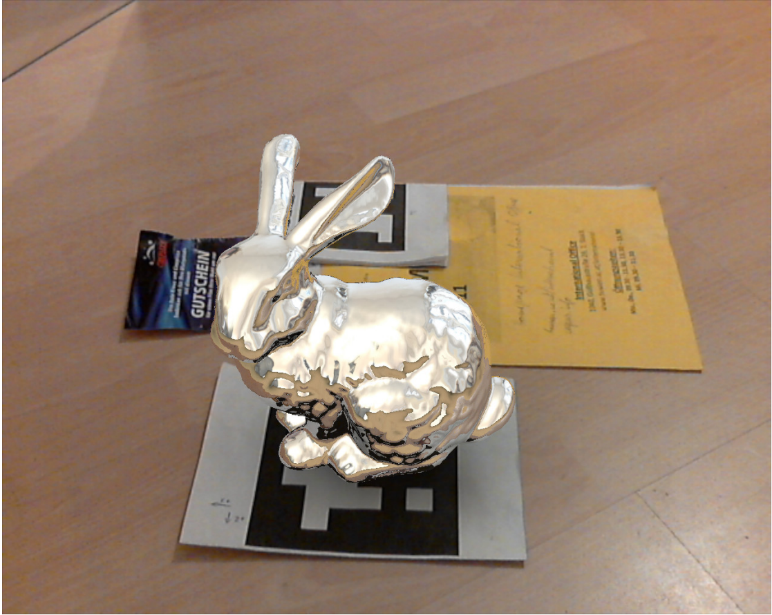
Figure A.5: Rendered with rasterization, 1280 x 1024, no AA, 7.2 fps
