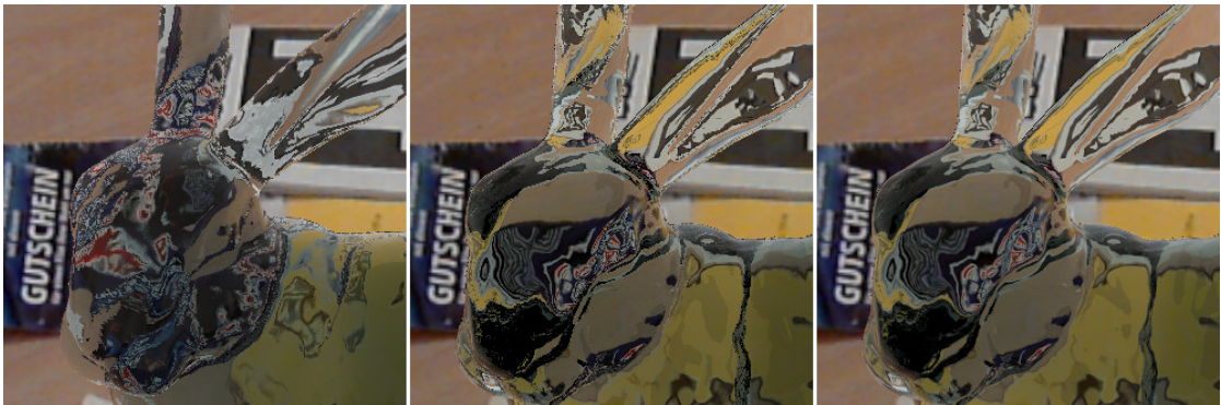
Figure 6.2: Left: Rasterization. Middle: Ray tracing without anti-aliasing. Right: Ray tracing with 9x SSAA.
