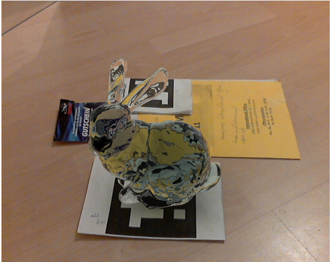
Figure A.3: Rendered with ray tracing, 1280 x 1024, 4x SSAA, 0.8 fps
