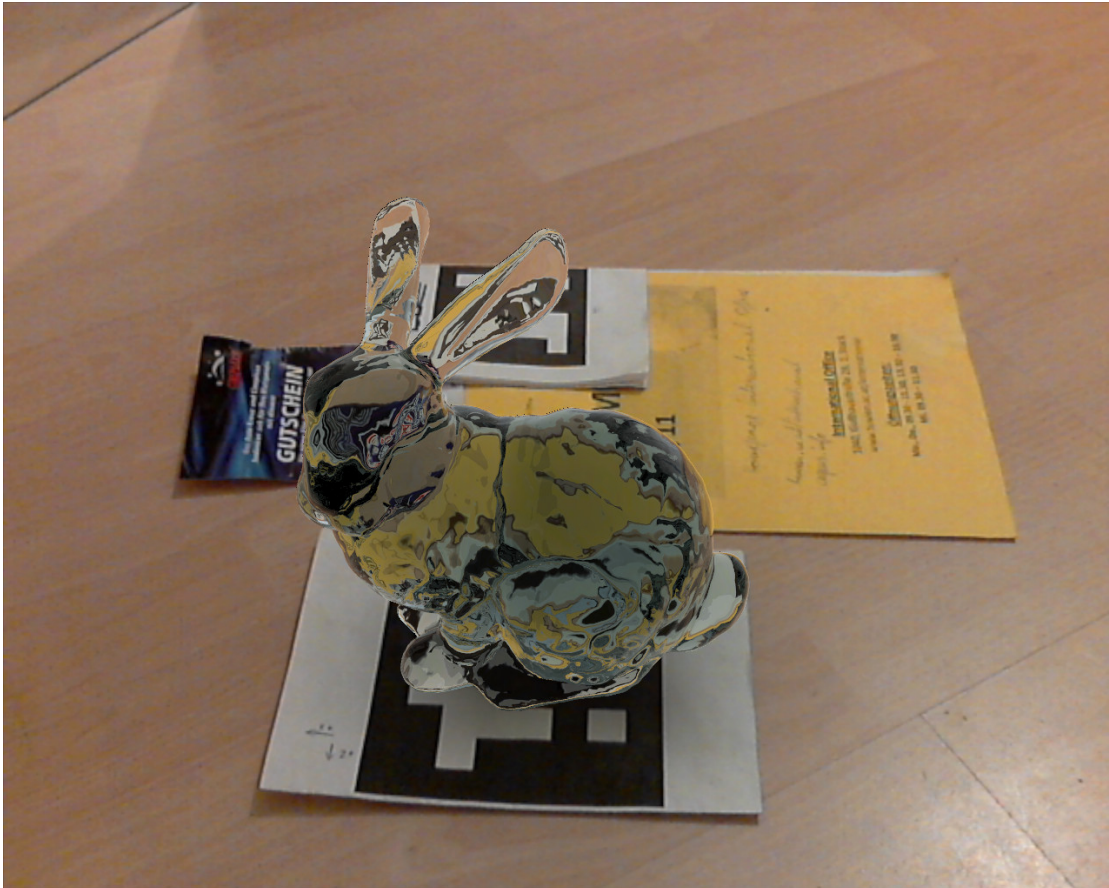
Figure A.4: Rendered with ray tracing, 1280 x 1024, 9x SSAA, 0.5 fps
