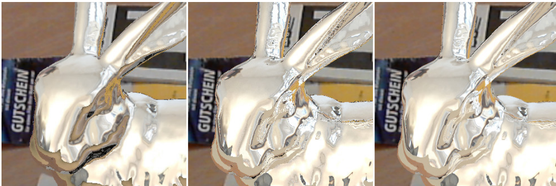
Figure 6.4: Left: Rasterization. Middle: Ray tracing without anti-aliasing. Right: Ray tracing with 9x SSAA.
