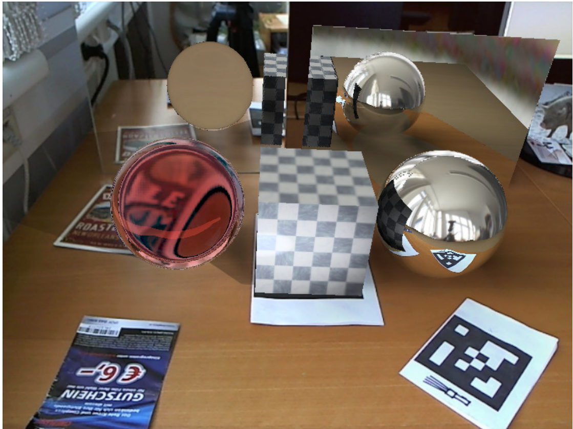
Figure A.11: Rendered with rasterization on PC 2 (see Chapter 6.1), 800 x 600, no AA, 17.2 fps
