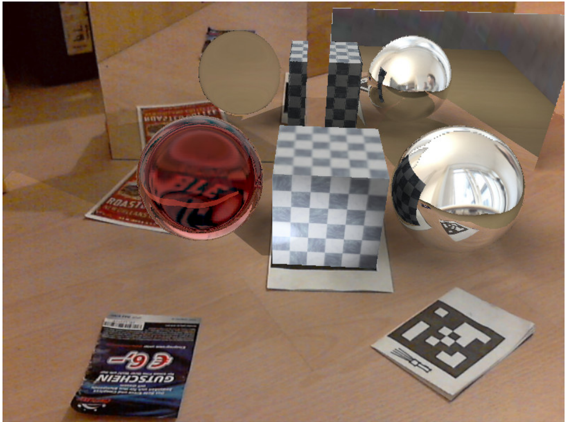
Figure A.9: Rendered with rasterization, 800 x 600, no AA, 10.2 fps
