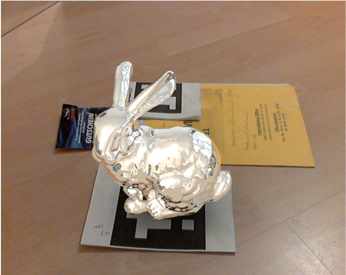
Figure A.7: Rendered with ray tracing, 1280 x 1024, 9x SSAA, 2.3 fps
