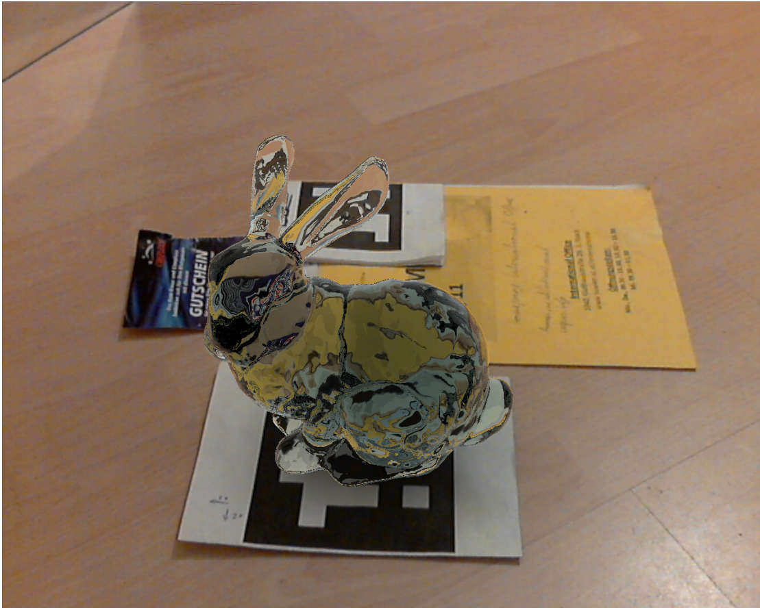
Figure A.2: Rendered with ray tracing, 1280 x 1024, no AA, 3.1 fps
