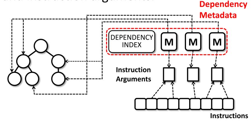
This allows the system to update the render cache **incrementally** as long as the structure of the scene graph does not change. This way **animated scenes** containing moving objects can be cached too.
