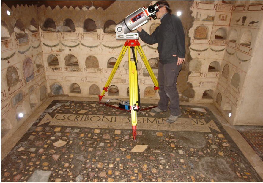
Figure 1.1: RIEGL VZ-400 laser scanner with top mounted Digital SLR. Image taken from [14].
