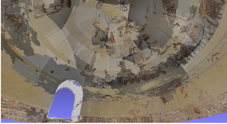
Figure 3.2: Result of the labeling using the best fragment approach. Every face is textured by the “best” photo, which leads to many seams.
