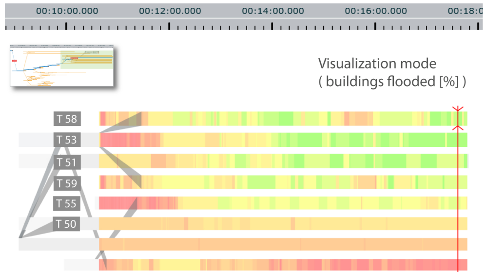
Figure 2.24 – Visualization mode that analyzes the percentage of flooded buildings using a combined current time-step and frame-wise visualization of all tracks that were investigated during the refinement and stability-test stages.
