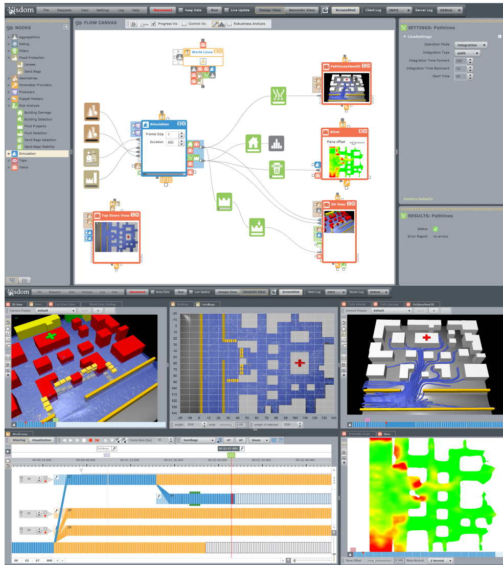
Figure 6.1 – Visdom [2] integrates simulation, steering and visual analysis into a unified, modular application. At its core is a data-flow network that is controlled by World Lines to enable interactive decision making.
