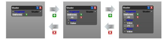
Figure A.18: Example of the growing ports mechanism. Everytime the *Add* icon is triggered the patch adds a set of input ports (Name, Value) to the *Uniforms*. In this example it was triggert twice. Clicking on the *Remove* icon removes just the set the icon belongs to.
