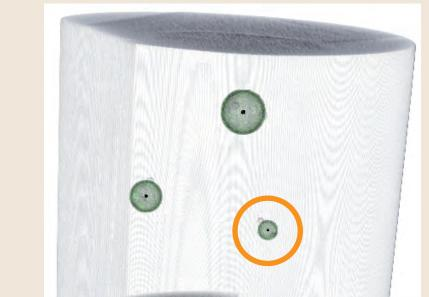
The information of the tracking paths is summarised to form the final result. The available cluster positions are marked in different colours, based on their occurance across the series of test castings.
