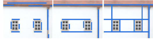
Figure 4: Nearly collinear line segments are merged and subsequently connected to form a grid.
