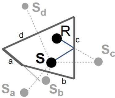
Figure 26: Image source method: with sound source  $S$  and virtual sound sources  $S_a, S_b, S_c, S_d$  [Funkhouser et al. 2002].
