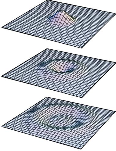
Figure 24: Application of the 2 dimensional waveguide mesh for transversal wave propagation in a membrane.
