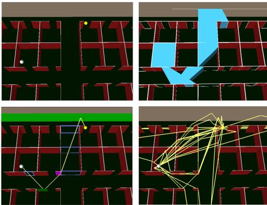
Figure 29: Beam tracing: a) scene with source (white) and receiver (yellow), b) traced beam in cyan, c) path generated for one beam, diffraction is visible at the cyan part of the beam d) paths for all possible beams (there are more than one) [Tsingos et al. 2001b].
