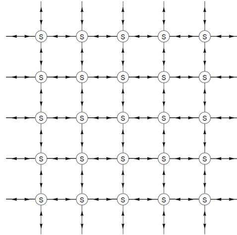
Figure 23: 2 dimensional waveguide mesh. Junctions S are connected with waveguides
