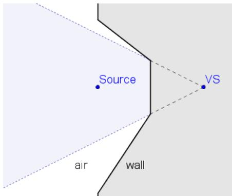
Figure 27: Visibility for the image source method. The listener inside the blue shaded region can hear the virtual sound source VS.
