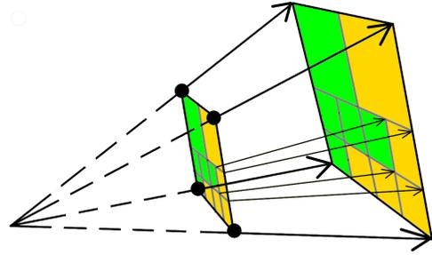
Figure 31: Frustum tracing casts volumetric frusta into the scene. These can only be split and merged in frusta with quadratic front and back planes.
