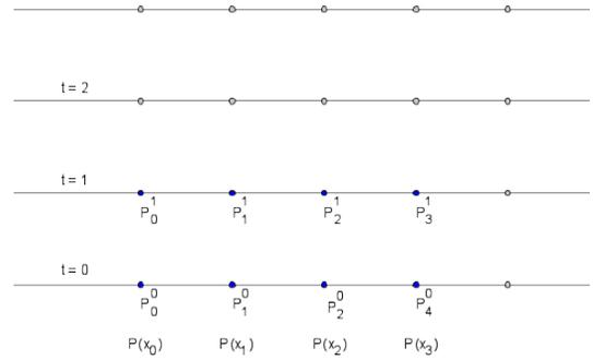
Figure 21: FDM for a one dimensional case. The horizontal lines can be imagined as a real physical object. The vertical axis symbolizes the time steps.
