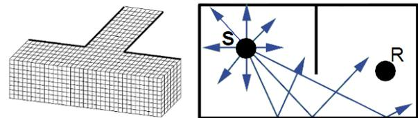
Figure 1: left: A numerical method discretizing space in cubes, right: Geometric ray casting with a source S and a listener R
