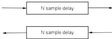
Figure 22: Digital waveguide
