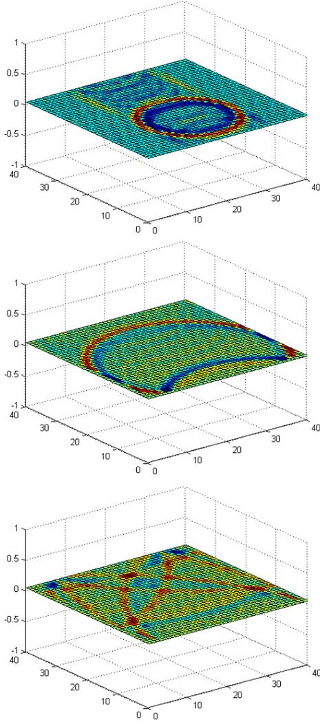
Figure 20: 2D rectangular wave propagation simulation in Matlab.
