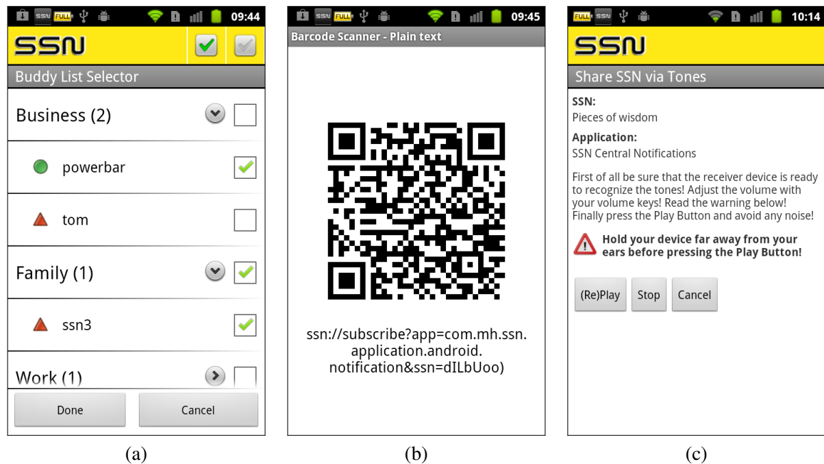
Figure 5.4: The activities for sharing an SSN with the help of invitations (a), visual codes (b) and tones (c): The user must select the buddies that should be invited to an SSN (a). (b) shows the activity of the Barcode Scanner from the ZXing Team [Zxi11] that displays the QR Code to share an SSN. In (c) the playing of the SSN tones can be started, stopped and restarted.
