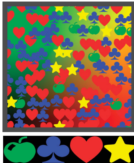
Figure 2.26: Four images stored in a texture map (bottom), which are irregular and randomly tiled over a single texture using texture bombing.
