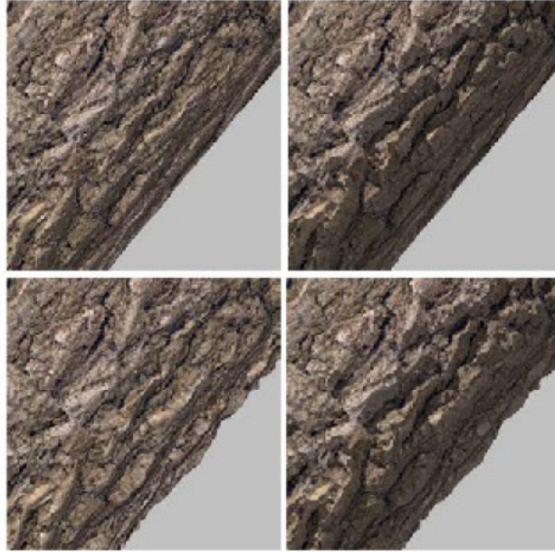
Figure 2.12: Comparison of different mesostructure rendering techniques. Bump mapping (top left), horizon mapping (top right), displacement mapping (down left) and view-dependent displacement mapping with self-shadowing (down right). [2]
