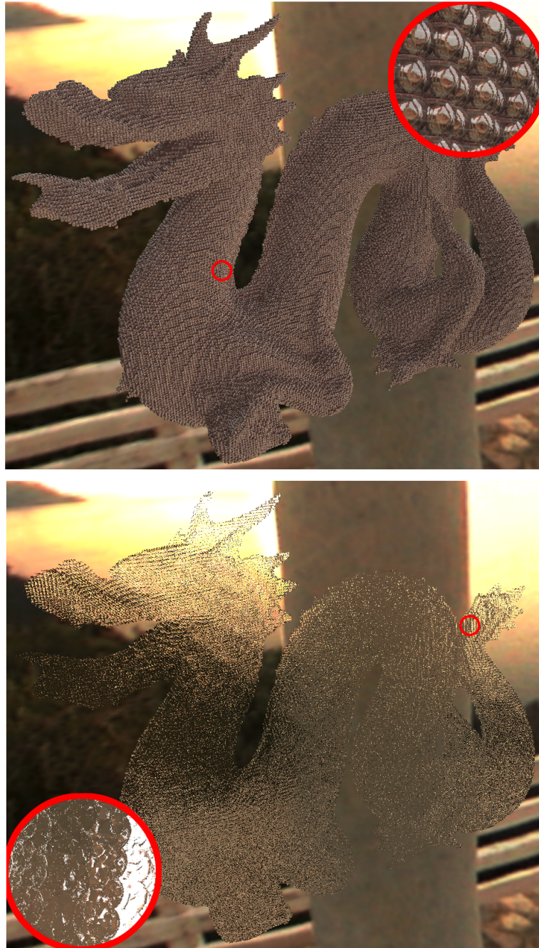
Figure 5.8: A cell-based dragon model rendered with specular self-reflection (top) and refraction (bottom). The cell dimension is 64 \times 64 \times 64 and the object space is split into 128 \times 128 \times 128 tiles. The color texture is taken from [23] .
