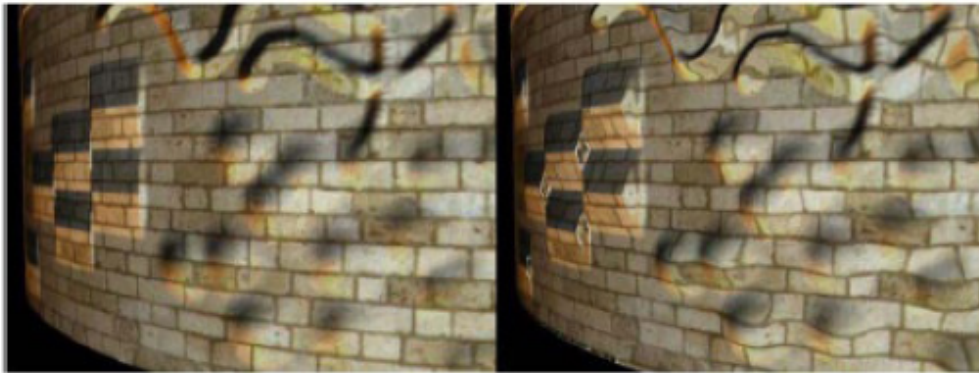
Figure 2.7: Wall rendered with bump mapping (left). Same wall rendered with parallax mapping (right). Note the parallax effect at the house tops' side walls on the left side of the brick wall. [9]
