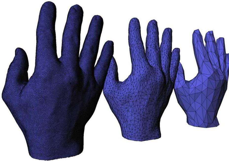
Figure 1.1: Illustration of Simplification. Image taken from CGAL Manual [6]
