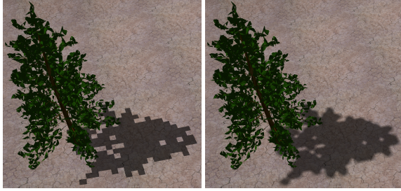
Figure 22: Undersampled unfiltered shadow maps on the left suffer from hard jagged edges. These can be removed by filtering. On the right hardware PCF with a 2x2 kernel is applied.
