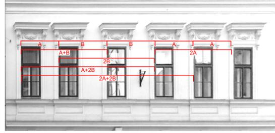
Figure 9: Demonstration of a number of possible multiples of offsets  $A$  and  $B$  which might obscure the results of the histogram extraction. Two, three and four times multiples of an offset happen quite often and can be easily removed by postprocessing.
