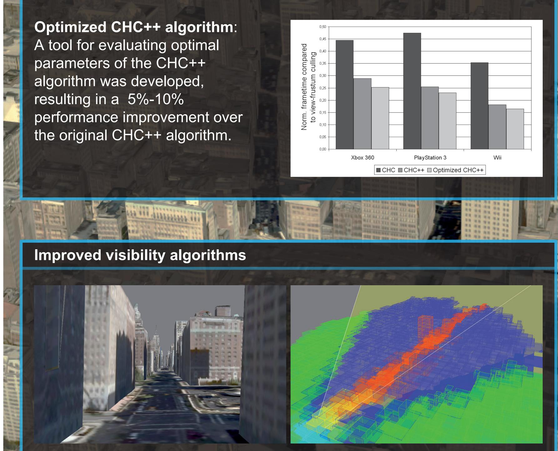
**Left**: Camera viewpoint. **Right**: Visibility visualization. Visible objects must be rendered, while occluded objects are discarded. The used visibility algorithm is able to cull about 80% of all objects in the scene in this case.
