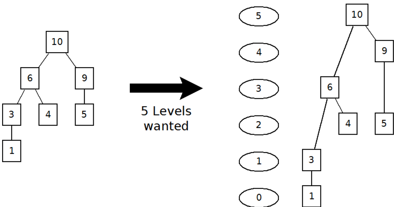
Figure 7: The 'OBB, ...' level mode. For each node a value v is calculated (how this value is calculated is based on which 'OBB, ...' is selected), then the Wanted # Levels are used to calculate the level value for each node by interpolating the v values.
