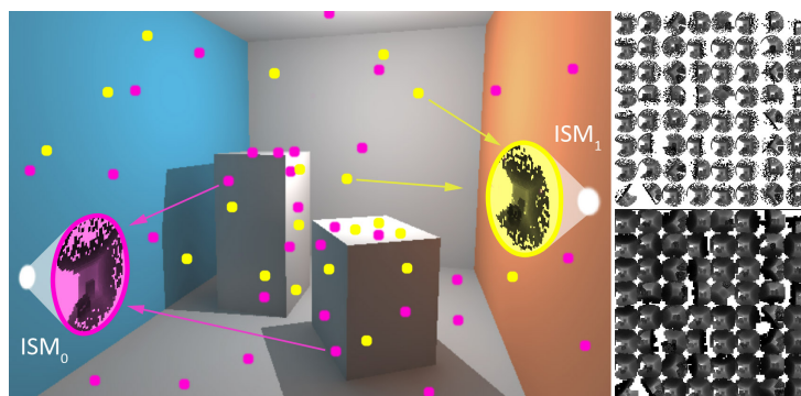
Figure 2.21: (left) Imperfect shadow maps [RGK*08] utilize a coarse point based representation of the scene (pink and yellow VPLs use only the pink and yellow points, respectively). (right) Imperfect shadow maps generated in a single frame. (top) With and (bottom) without push-pull algorithm for repairing the holes (Image courtesy of Ritschel et al. [RGK*08]).
