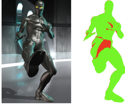
Figure 2.31: Even for quickly moving objects, most pixel information from the previous frame can be reused in the current frame (shown in green) and only some parts have to be recomputed (shown in red) (Image courtesy of Nehab et al. [NSL*07]).
