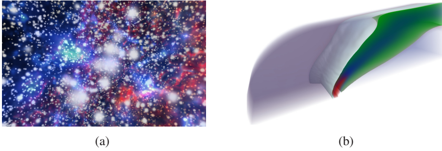
Figure 1.8: Visualization of non-uniform point sets with hybrid approaches: a) astronomic data rendered with a hybrid ray caster [51], and b) simulation data rendered with a ray caster adopted to MLS [58].
