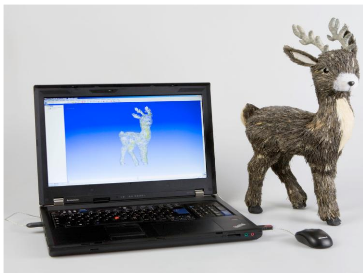
Figure 3 The laptop with the raw point cloud after scanning and the scanned model aside of it.
