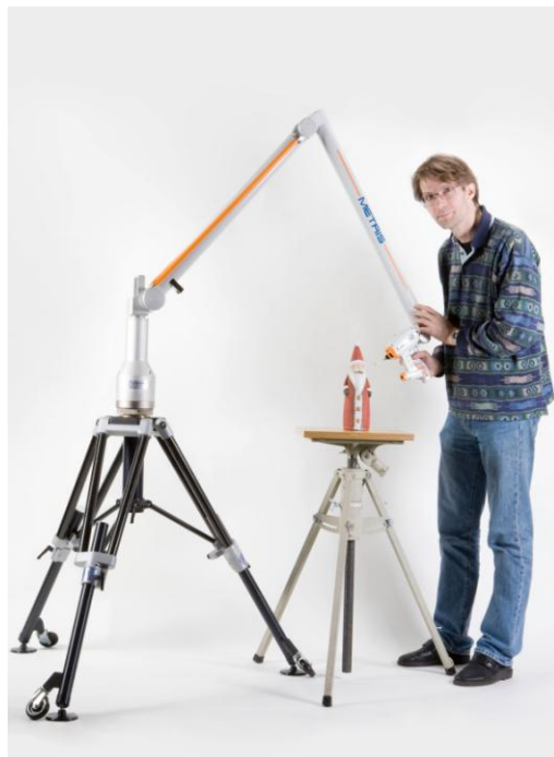
Figure 2 The setup of the scanning arm at the laboratory of the Institute of Art and Design at the VUT.
