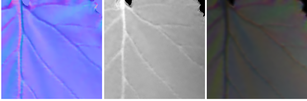
Figure 3.16: The normal map, height map, and the resulting HL2 coefficient map.
