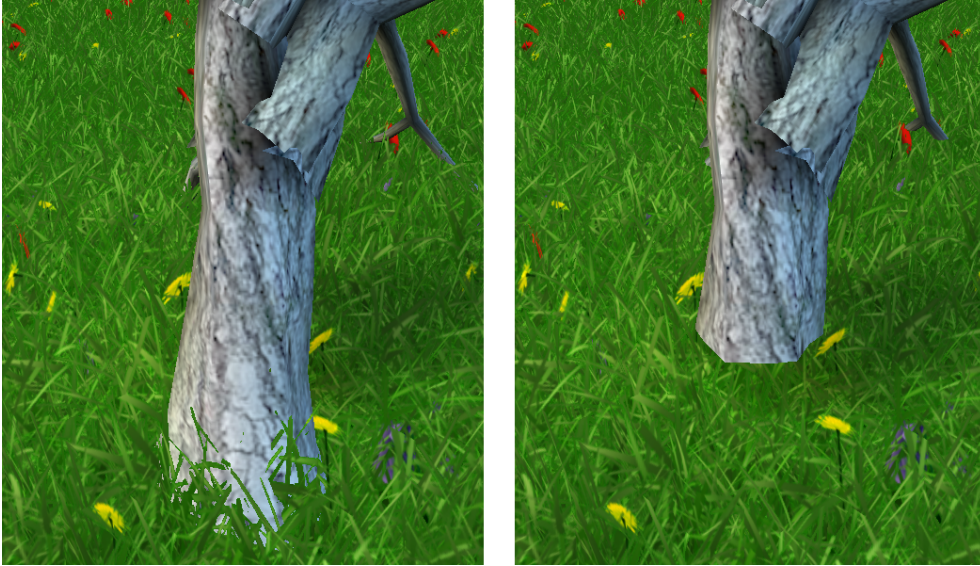
Figure 2.14: A grass patch with (left) and without (right) correct visibility.
