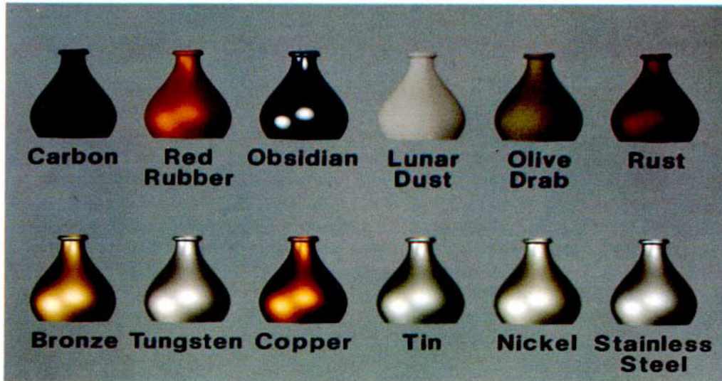
Figure 2.7: Several materials simulated with the Cook-Torrance reflectance model (image taken from [CT82])
