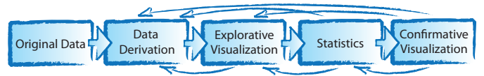
Fig. 2. Interactive visual exploration of climate data: Meaningful climate parameters are derived from the original data which are explored interactively in order to form hypotheses. Statistical analysis confirms or rejects the hypotheses. The results from analysis are generally visualized for illustration. In this pipeline each step can also reflect back on previous steps for efficient information drill down.
