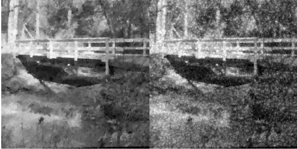
(a) tvqc, k = 0.1l , PSNR=22.56, time=1213.91s (b) hierlsqr, k = 0.1l , PSNR=20.45, time=12.64s
