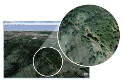
Figure 1.1: Orthophotographic maps projected onto a terrain model become apparently 'flat' when viewed at low angles.
