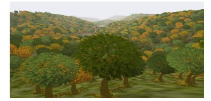
Figure 2.9: Sample scene rendered using *Deferred Splatting* [GBP04]. The scene contains approximately 2300 visible trees consisting of approximately 750k polygons each. It is rendered at 11fps.
