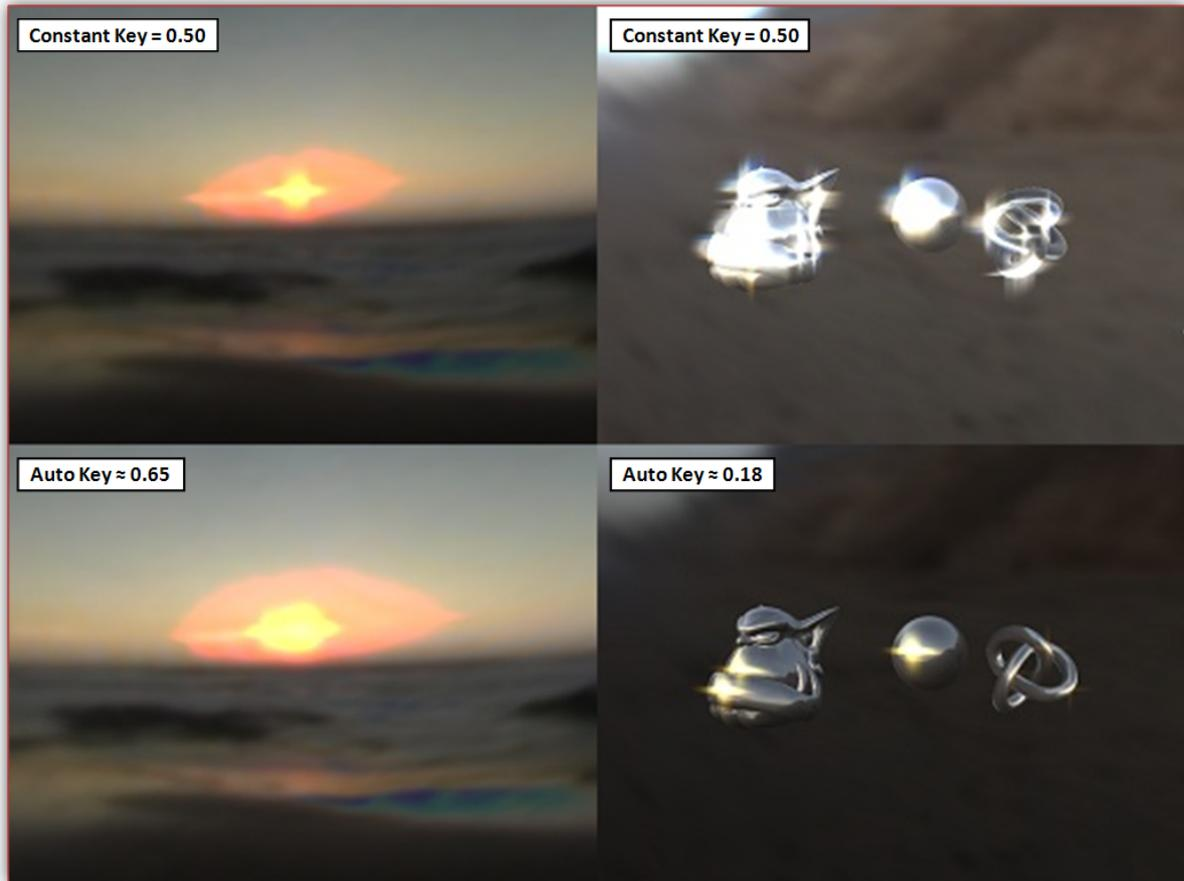
Figure 7: Showcase of the automatic key calculation in comparison to a constant key.
