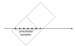
Figure 9: A ray is propagated to the adjacent brick it enters after it is processed for the active brick. To achieve this, the entries of the corresponding brick arrays  $brick\_fromRay$  and  $brick\_toRay$  are updated.
