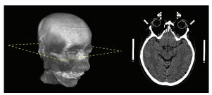
Figure 1: To generate an MPR-slice, a plane is defined which intersects the volume (left). Interpolated data values are shown on this plane (right).
