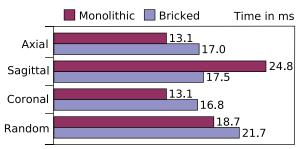
Figure 10: The averaged time in milliseconds which is needed to compute one MPR image for the axial, the sagittal, the coronal and the random case.
