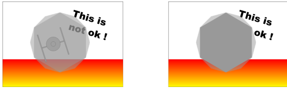
Figure 1: A spherical object in transition between two LODs that project to a 6- and 12-sided polygon in screen space respectively. In the background are a spaceship, a planet surface and a text object. Left: Conventional blending leads to semitransparency during the blend, making objects behind the LOD object visible—the player could wrongly see the spaceship. Right: In our new method, one of the LODs is drawn opaquely, solving the transparency problem.
