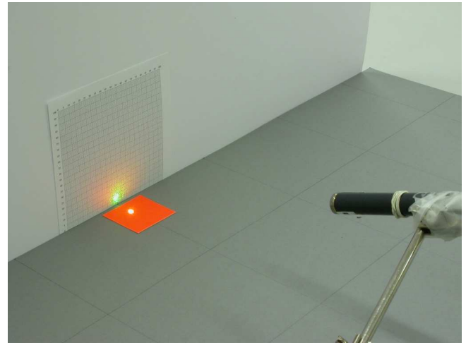
Figure 2: Overview of the experimental setup. Since our aim was just to provide a qualitative visualisation of the phenomenon we are trying to represent, we used a comparatively simple setup: a green handheld laser pointer (wavelength 532 nm) fixed to a mount, material samples 4 \times 4 cm in size, and a small grid printed on diffuse white paper as target for the reflection pattern. The scene was captured with a Nikon 4500 digital camera, which offers the possibility to manually control all relevant parameters such as aperture and shutter speed.
