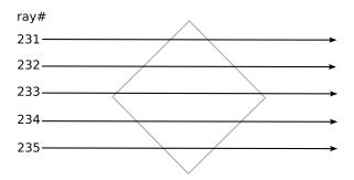
Figure 7: The brick is intersected by a number of rays. Two *brick\_fromRay* and *brick\_toRay* arrays keep track of this by storing the number of the first and of the last ray.
