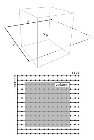
Figure 5: The point p and vectors u and v define the MPR plane in object space (top). This plane is mapped to the image space and rays are cast through the volume (bottom). The volume is resampled along these rays.
