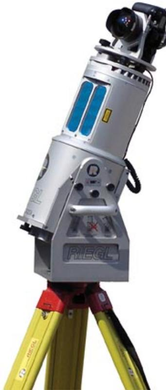
Fig. 1.1: An example of a terrestrial laser scanner. Here a Riegl LMS z420i is shown. The range measuring laser is situated behind the blue windows in the scanner's casing. After taking range samples from the environment, the camera on top of the scanner takes photographs of the scanned environment.
