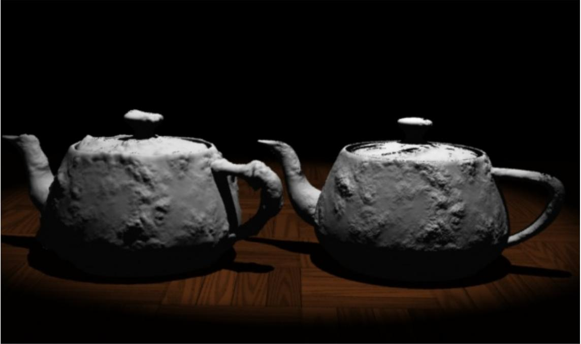
Figure 2.4: Two effects created using programmable shaders. On the left, the teapot is rendered using displacement mapping, which simulates surface structures without adding geometry. On the right, simple bumpmapping is used. Note how the illusion of the ripples is lost at the silhouette of the right teapot, whereas displacement mapping distorts the silhouette as well.
