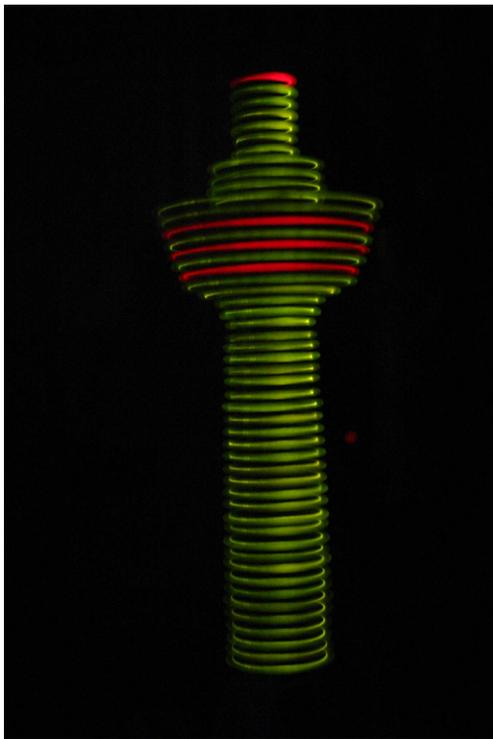
Figure 16: A volumetric display made of rotating leds
