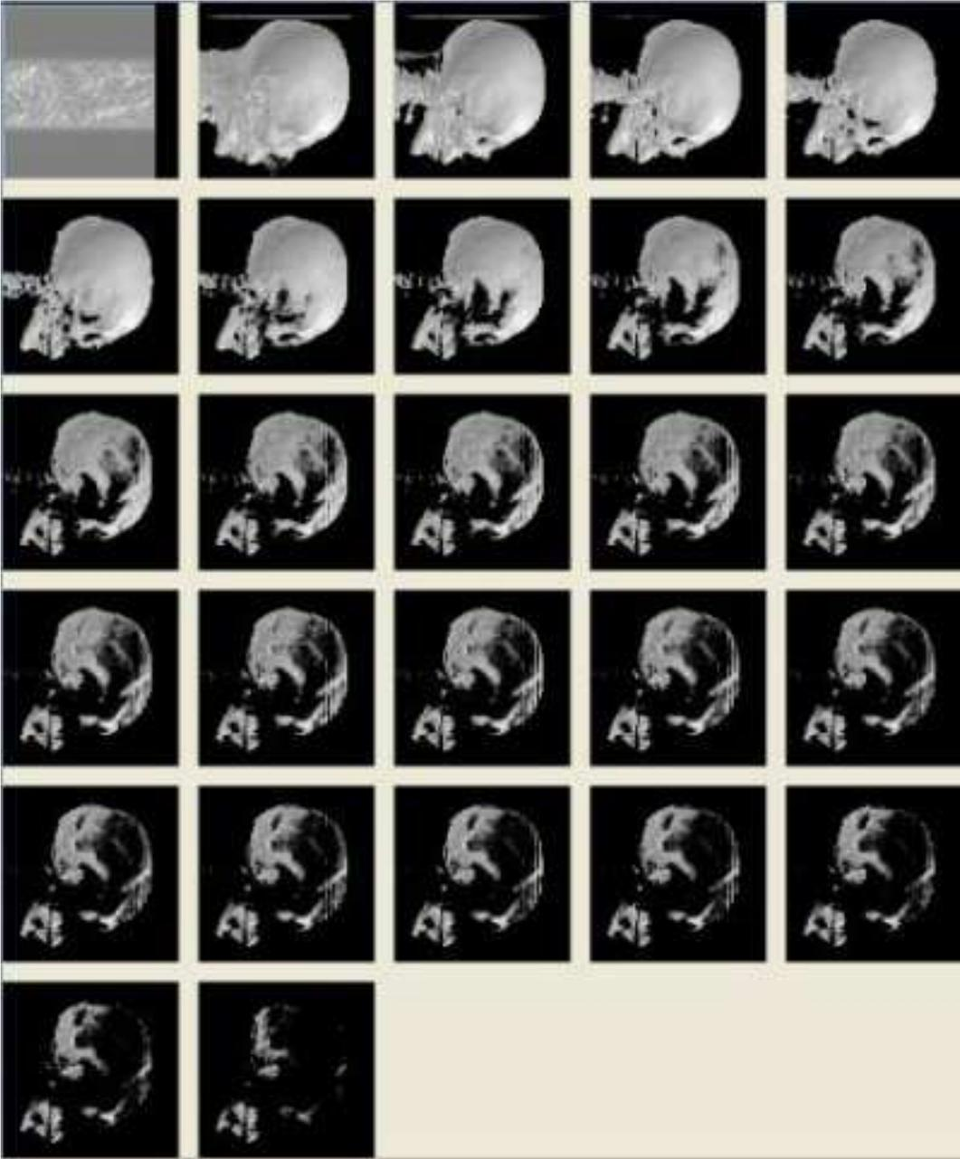
Figure 3.9: Result of Local Maxima Method: Here the local maxima method was combined with the pixel-difference method (Section 3.2.4) with a threshold value of 2500
