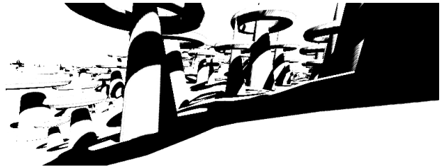
Figure 7: The shadow map is applied to the unlit and uncoloured geometry.
