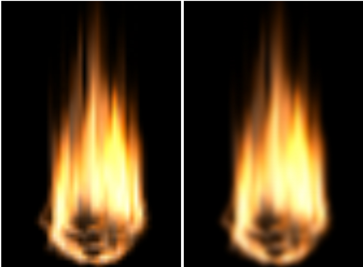
Figure 3.18: Pre-rendered 2D texture animation of a flame. (left) bi-linear interpolation; (right) filtering with bi-cubic B-spline. The left image exhibits many interpolation artifacts especially at the base of the flame, and vertical line artifacts at the top.
