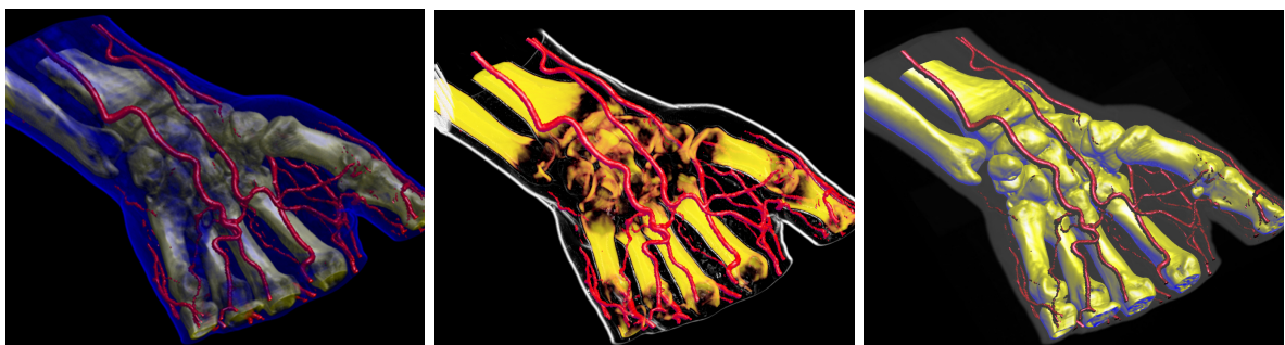
Figure 7.4: Segmented hand data set (256x128x256) with three objects: skin, blood vessels, and bone. Two-level volume rendering integrates different transfer functions, rendering and compositing modes: (left) all objects rendered with shaded DVR; the skin partially obscures the bone; (center) skin rendered with non-photorealistic contour rendering and MIP compositing, bones rendered with DVR, vessels with tone shading; (right) skin rendered with MIP, bones with tone shading, and vessels with shaded isosurfacing; the skin merely provides context.
