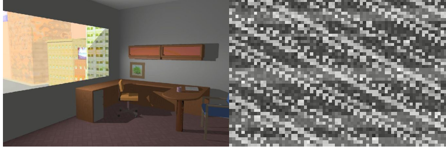
Figure 6.3: The input image and the luminance samples. (left) The input image (1000x700 pixels). (right) Filtered Random sampling (1024samples).
