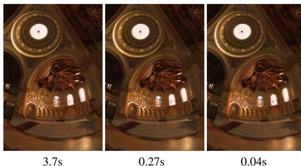
**Figure 1:** (left) Image tone mapped using the operator of Pattanaik et al.; computational time 3.7s. (center) Result of a software implementation of the proposed technique using the same tone mapping operator (0.27s). (right) Result of the hardware implementation (0.04s).
