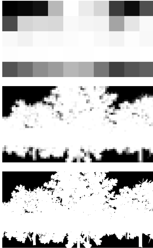
Figure 5.7: The hierarchical occlusion map represents the occlusion in the image hierarchically at several resolutions.
