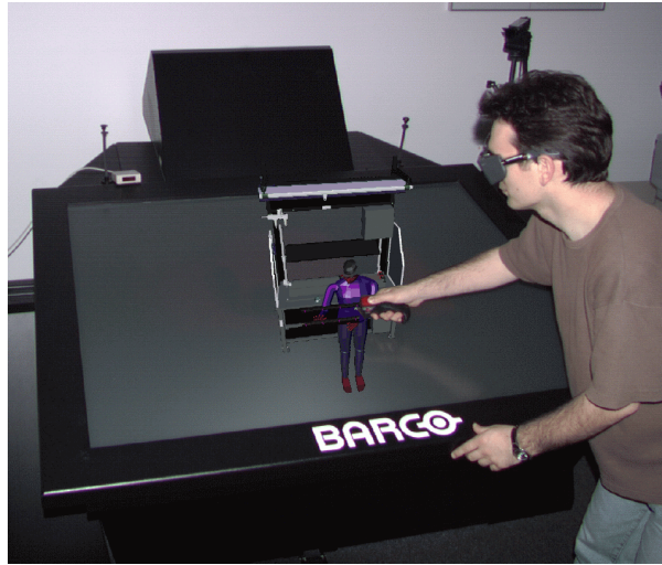
Figure 6.1: The responsive workbench environment – objects are perceived as being above the display surface
