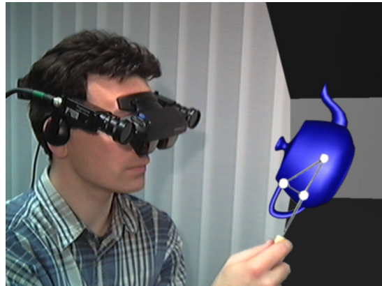
Figure 6.14: See-through HMD for inside-out tracking
