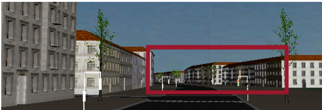
Figure 5.1: A scene from an urban walkthrough. Geometry in the red region has been replaced by a point-based impostor, providing for fast, antialiased rendering of the far field.
