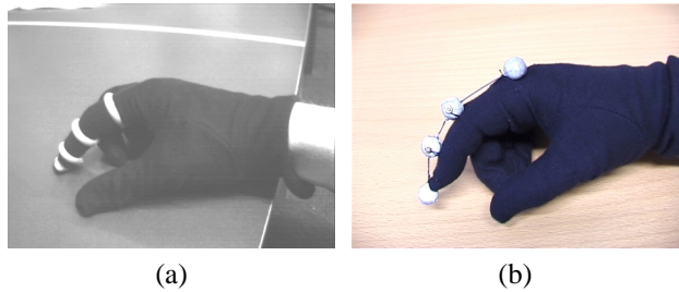
Figure 4. Gloves fitted with retroreflective markers
