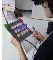
Figure 1: Working with the PIP in augmented reality. By looking out from underneath the head mounted display at the menu panel, the instructions on a sheet of paper can be read (left), by looking through the HMD the menu system with 3D buttons can be seen (right).
