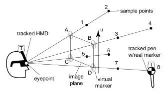
Figure 4: geometric determination of HMD parameters
